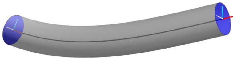
Figure 2: Schematic of a geometrically exact beam. Two exemplary cross sections are shown, through which the central line \mathbf{r} (black) passes. Also shown are the three director vectors \mathbf{d}_1 (cyan), \mathbf{d}_2 (white), \mathbf{d}_3 (red).
