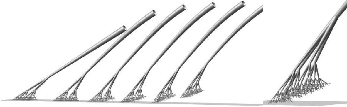
Figure 4: Pull-off of a gecko seta with v = 0.1 m/s. The six configurations on the left show the deformed seta structure at the pull-off displacements u = 0, 16, 22, 25, 27 and 30 \mu\text{m} . The enlargement on the right shows the deformed seta prior to jump-off, at 27 \mu\text{m}
