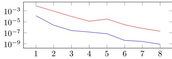
Fig. 2:  $\max_{\mu \in \mathcal{D}} \frac{\Delta_N(\mu)}{\|u_N(\mu)\|_V}$  and corresp.  $\frac{\|u(\mu) - u_N(\mu)\|_V}{\|u_N(\mu)\|_V}$ .
