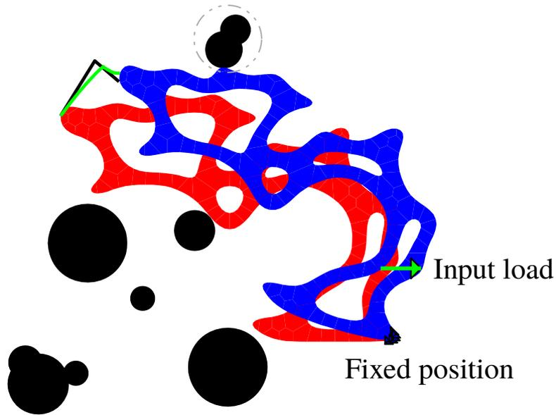
Figure 9: Undeformed (red solid), deformed (blue solid), contact surfaces (black solid), the desired path (black curve) and the actual path (green curve) are shown. Active contact surfaces are enclosed within dash-dotted circle.
