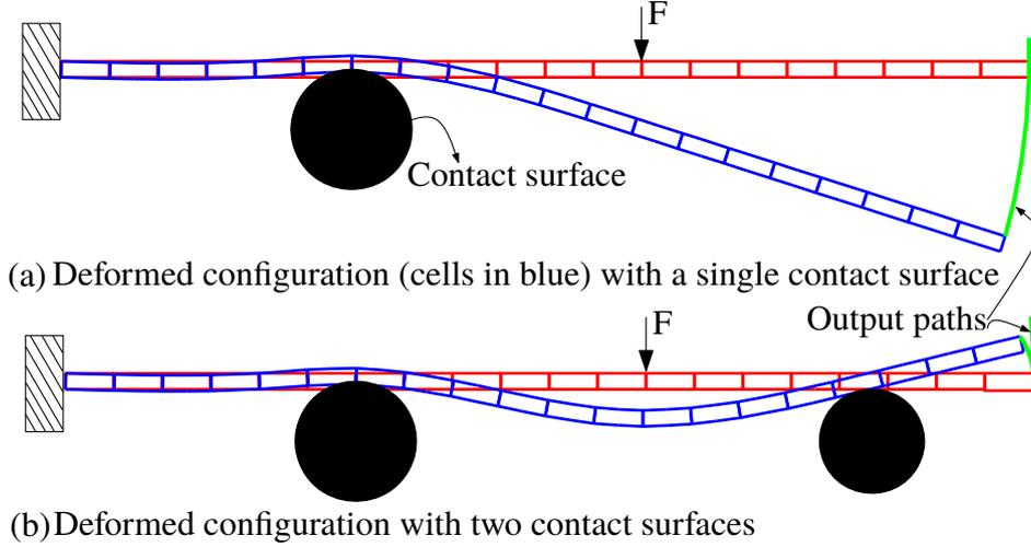
Figure 5: Example of single and multiple contact analysis with a cantiliver beam. Depending on nature of contact, back tracking (a) of the output port (the beam tip) or a kink (b) is observed.
