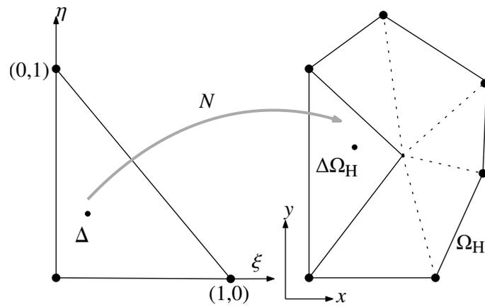
Figure 3: Each cell is divided into six subregions and integration over each subregion is performed to evaluate the element stiffness matrix  $\mathbf{k}$ .
