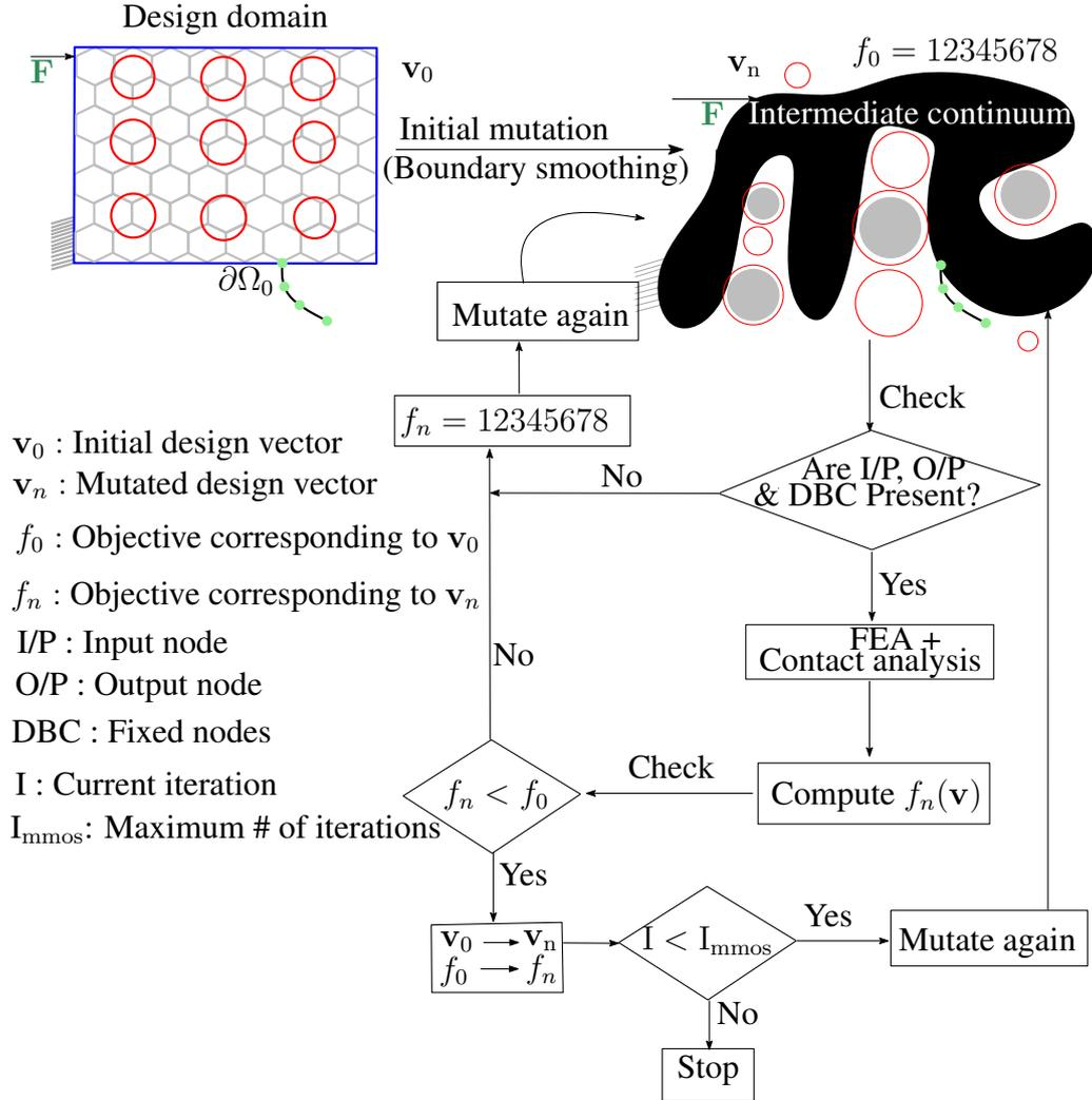
Figure 7:  $\Omega$  is discretized via hexagonal cells  $\Omega_H$ . Negative circular masks  $\Omega_M$  are employed to remove the material and to encompass contact surfaces within some. Contact analysis with minimization of Fourier Shape Descriptors based objective is performed to achieve the path close to that desired.
