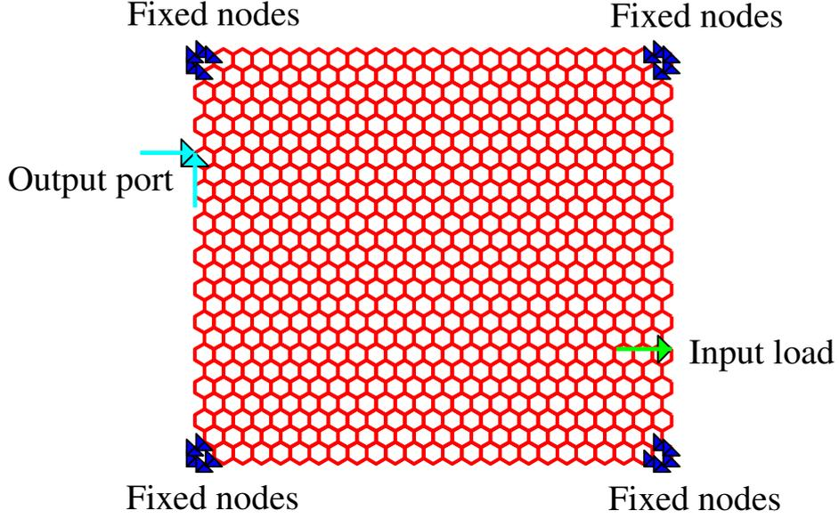
Figure 8: Design specifications for the synthesis of CCMs
