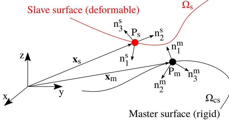
Figure 4: Contact formulation of the two bodies  $\Omega_s$  and  $\Omega_{cs}$  in their current configuration. Normal triad on  $P_s$  are  $\mathbf{n}_i^s$  and that on  $P_m$  are  $\mathbf{n}_i^m$ , where  $i = 1, 2, 3$ .
