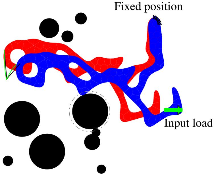
Figure 12: Undeformed (red solid), deformed (blue solid), contact surfaces (black solid), the desired path (black curve) and the actual path (green curve) are shown. Active contact surfaces are enclosed within dash-dotted circle.
