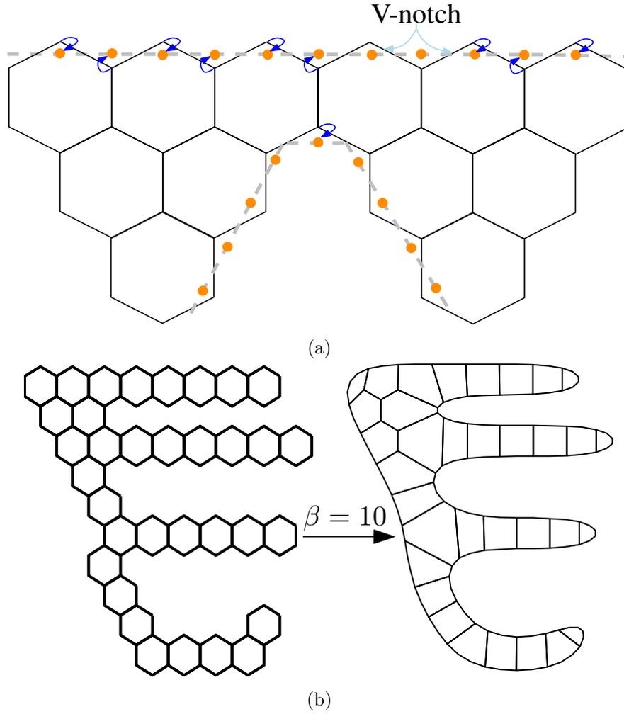
Figure 2: Boundary smoothing to facilitate contact analysis. (a) Mid-points of boundary edges are joined with straight lines and boundary nodes shifted along their shortest perpendicular distances on these segments. (b) Boundary smoothing with  $\beta = 10$  steps.
