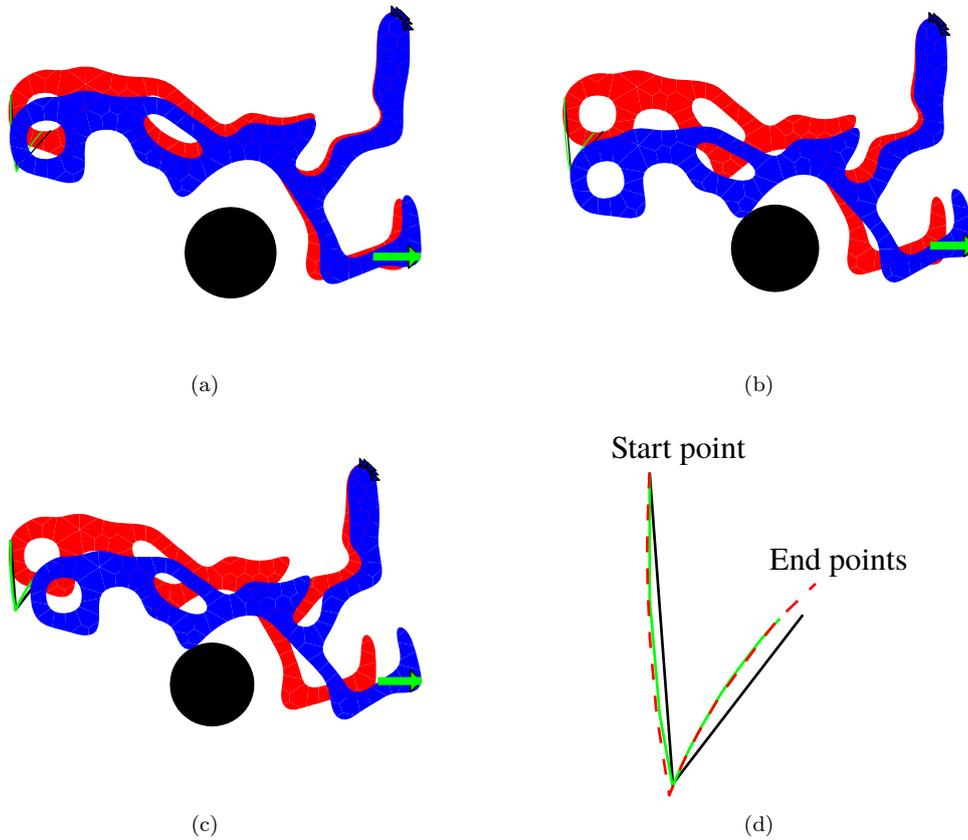
Figure 13: Different deformed configurations are shown in (a), (b) and (c). (d) shows comparison of the desired path (black), the actual path (green) and that using Abaqus (red dotted) with neo-Hookean material and 4 noded plane strain (CPE4I) elements.
