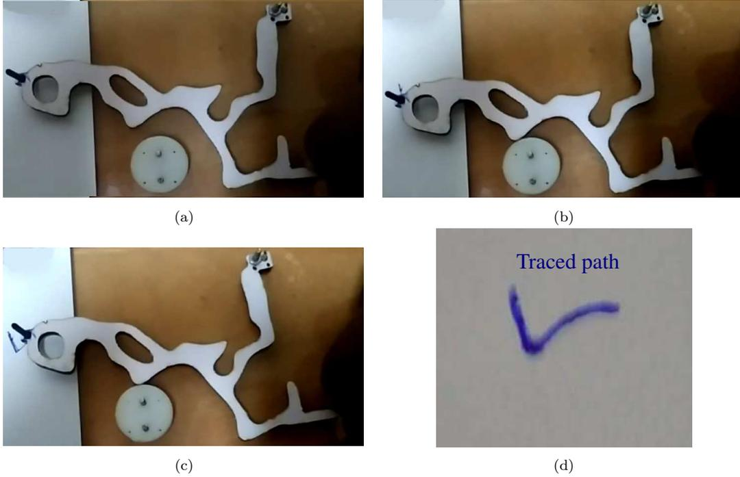
Figure 14: Different deformed configurations of the fabricated prototype for Example 2 are shown in (a), (b), and (c). (d) shows the traced path.
