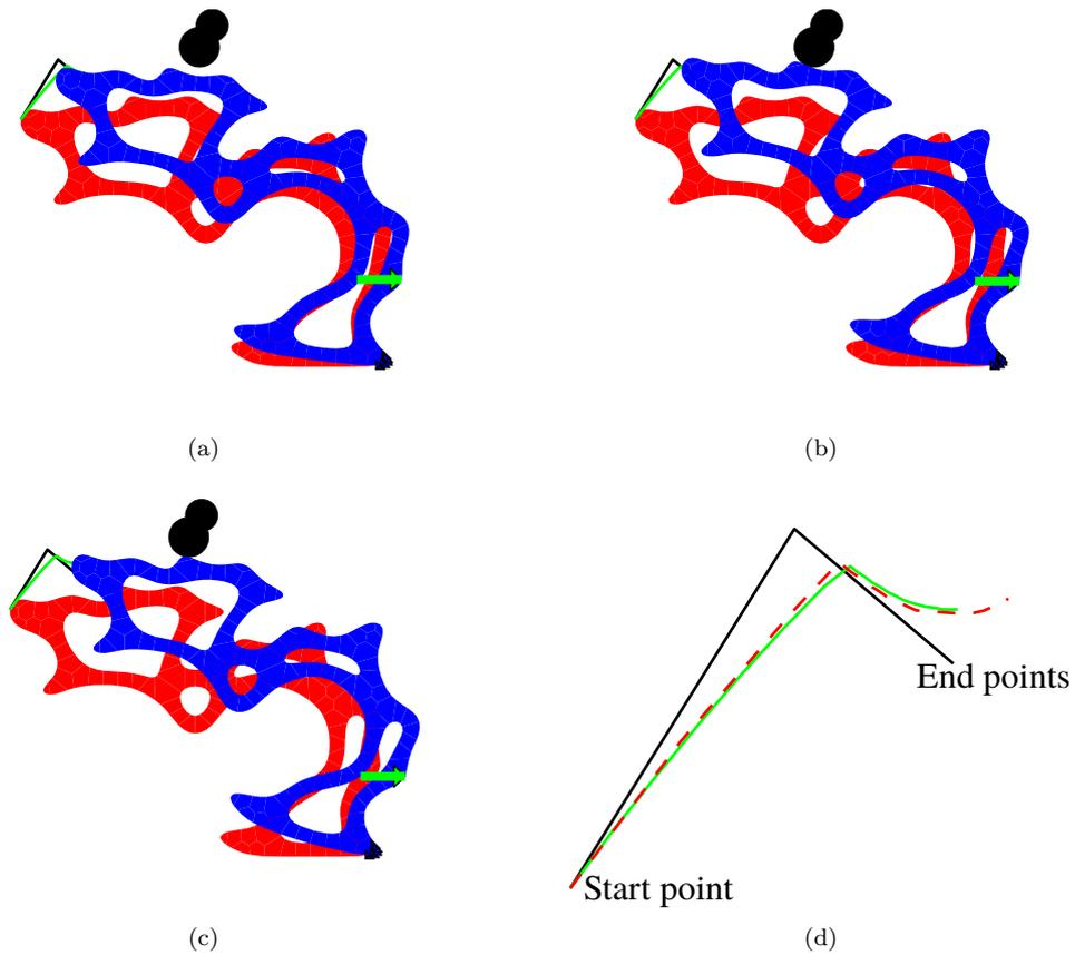
Figure 10: Different deformed configurations are shown in (a), (b) and (c). (d) compares the desired path (black), the actual path (green) and that using Abaqus (red dotted) with neo-Hookean material and 4 noded plain strain (CPE4I) elements.
