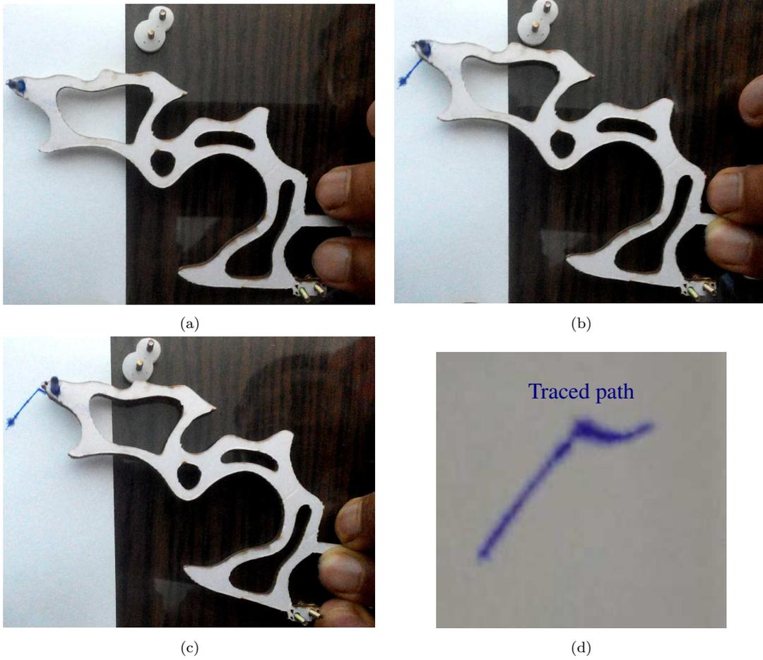
Figure 11: Different deformed configurations of the fabricated prototype for Example 1 are shown in (a), (b), and (c). (d) shows the traced path.
