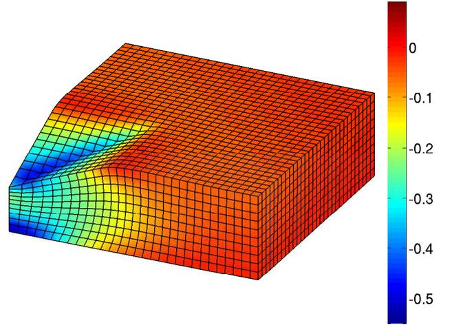
Figure 5: Nanoindentation of a rubber film: deformation and stress field under the indenter for weak adhesion ( $\gamma_W = 1000$ )
