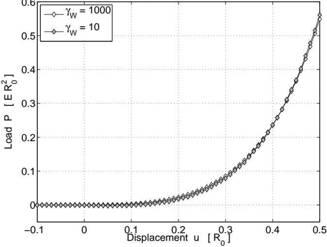
Figure 3: Load displacement curve  $P(u)$  for indentation with weak adhesion ( $\gamma_W = 1000$ ) and strong adhesion ( $\gamma_W = 10$ )
