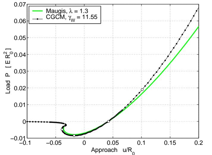
Figure 1: Load displacement curve for a sphere in adhesive contact with a half-space
