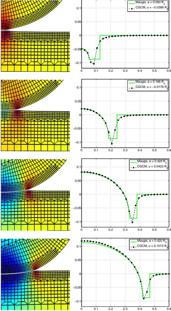
Figure 2: Contact between sphere and half-space: Deformation and stress field (left); contact pressure between the two bodies (right); The four cases correspond to the four states marked in figure 1.
