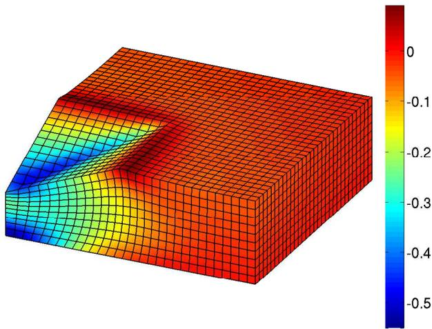
Figure 6: Nanoindentation of a rubber film: deformation and stress field under the indenter for strong adhesion ( $\gamma_W = 2.17$ )
