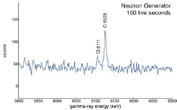
**Figure 5:** Gamma ray spectra for 14.1 MeV neutrons on oxygen, as obtained by A.J. Caffrey, INEEL, the sample was COCl<sub>2</sub> [19].
