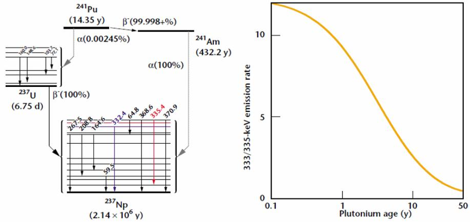
**Figure 2:** Left: The branching decay of Pu-241 shows the gamma ray transitions measured by the Pu300 method [2].
