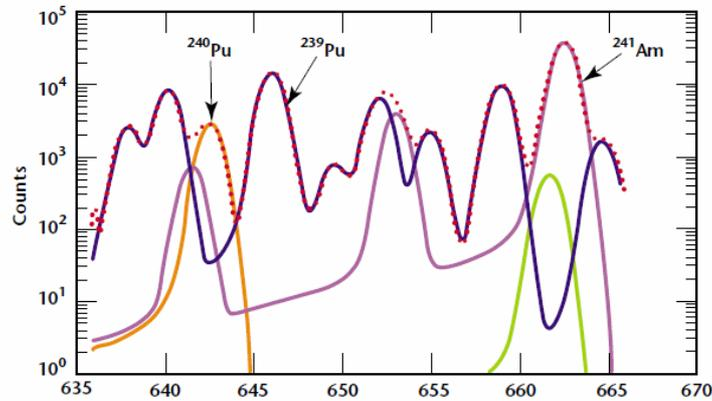
**Figure 3:** The 630-670 keV region of the gamma ray spectrum shows its resolution by nonlinear regression into its isotopic constituents for the Pu600 method [2]. The orange line corresponds to Pu-240, the light purple line to Am-241. The dotted line represents the total spectrum.
