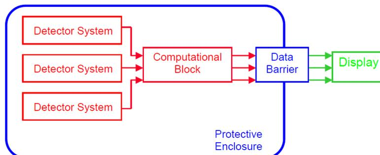
**Figure 1:** Attribute Measurement System with Information Barrier scheme that shows the attribute measurement detectors, the attribute-analysis computational block and the data barrier [5].
