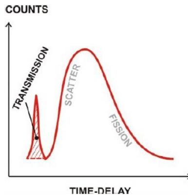
**Figure 4:** The integral of the first peak in the count-distribution is proportional to the neutron transmission rate and thus total uranium [19].
